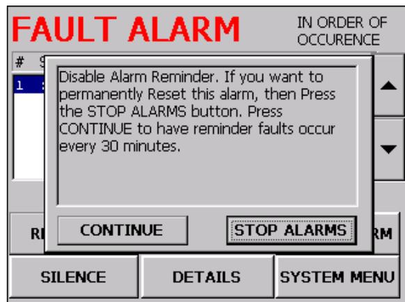
FIGURE 24.3 Select the reset function box.
