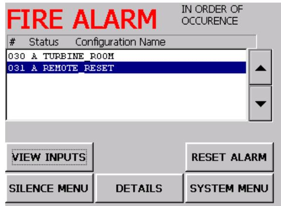
FIGURE 18.4 First, the turbine optical on node 0-1 was tripped, then the remote reset button on node 0-4 was pushed to reset the strobe.
