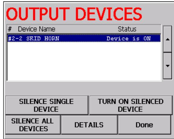
FIGURE 19.4 Silence menu selected indicating the horn is turned on.
