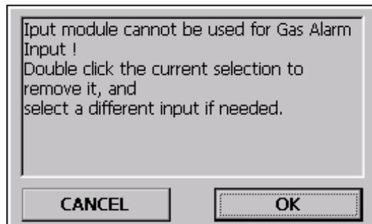
FIGURE 15.3 Error message when trying to select an input node for gas.
