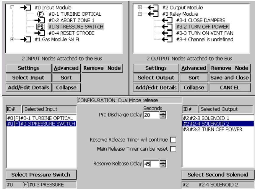
FIGURE 16.1 Input / output node mapping and selecting exceptions.
