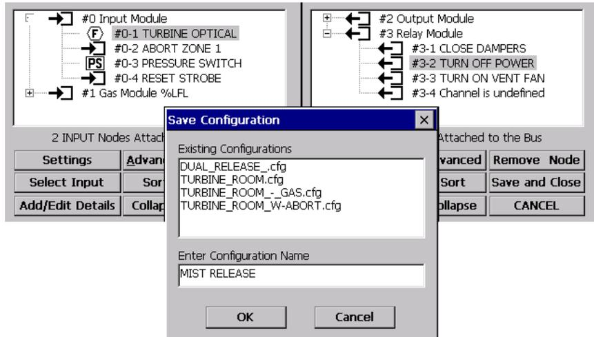
FIGURE 17.2 Naming the mist configuration.
