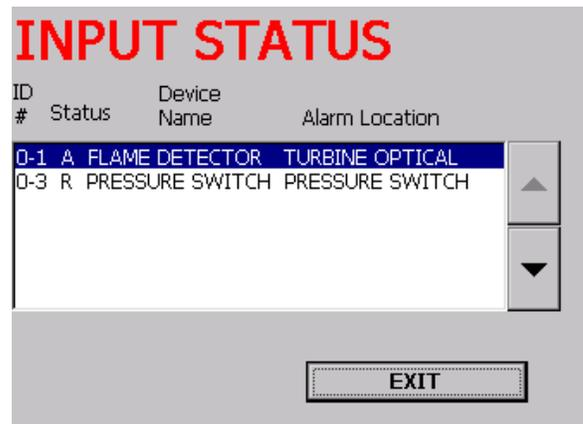
FIGURE 16.4 Input status menu indicating two alarm inputs from the configuration named “Dual Release”.
