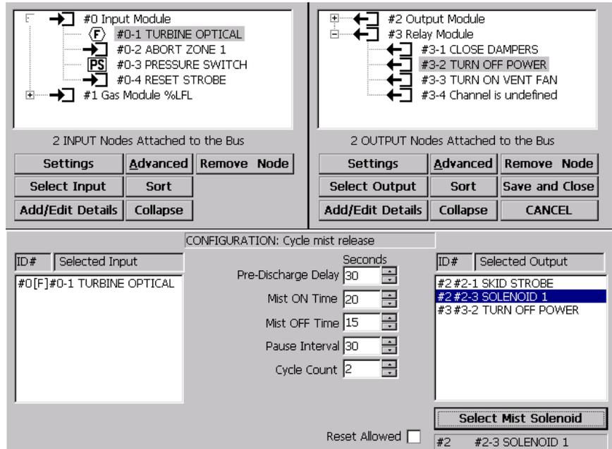
FIGURE 17.1 Selecting node channel inputs and outputs.
