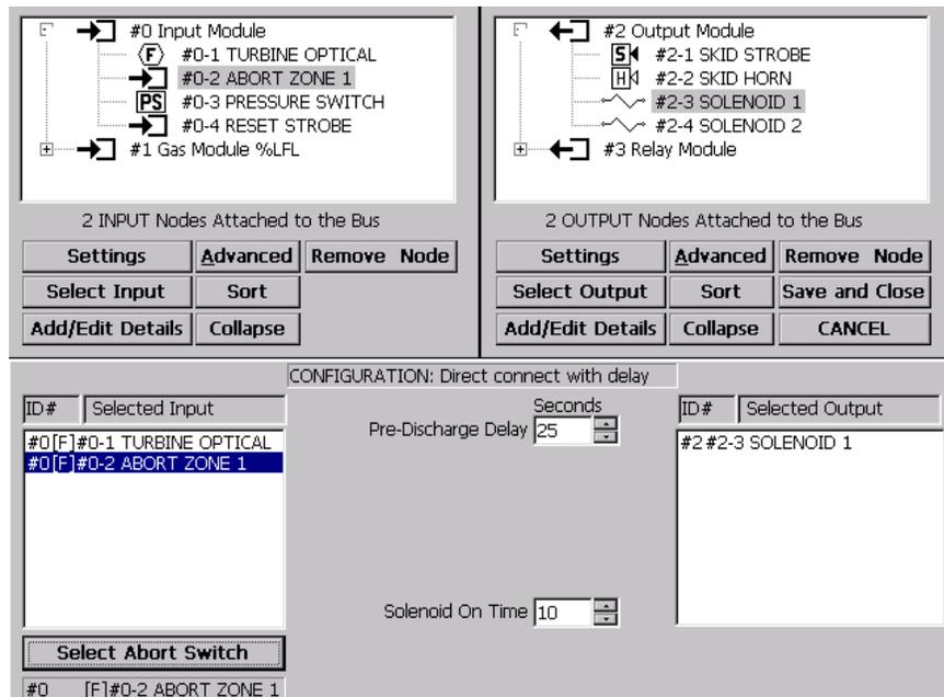
FIGURE 14.1. Loading the configuration with data.
