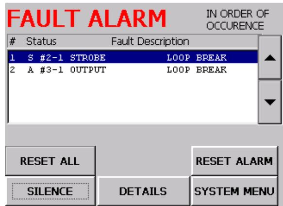
FIGURE 29.2. Loop break failure as described in sections 29.3.
