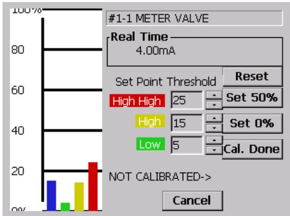
FIGURE 10.3 SET ZERO menu before SET 0% button is pushed with 4mA applied to input.
