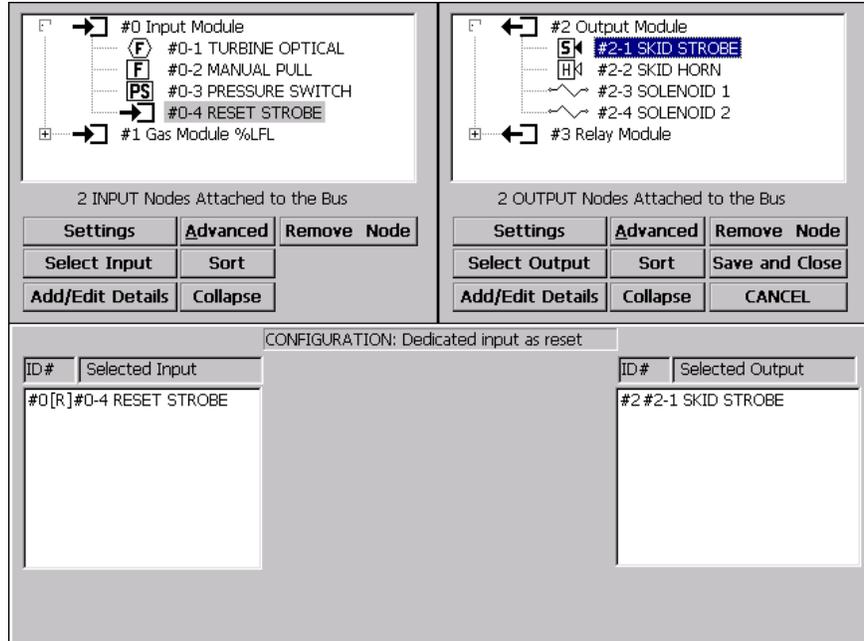
FIGURE 18. Dedicated Appliance Reset Configuration. Utilizing channel 4 of the input node to reset the strobe in the SELECTED OUTPUT. Channel 4 was named reset strobe back in the ADD/EDIT DETAILS in section 9 knowing it would be used in this example.
