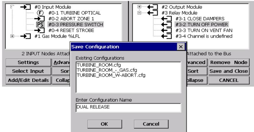
FIGURE 16.2 Saving the configuration. In this example the configuration file name is called “dual release”.
