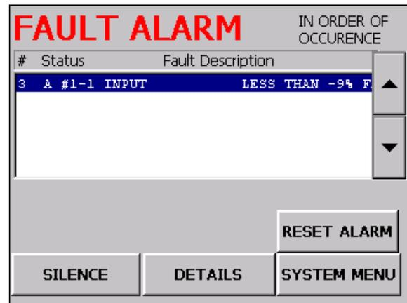
FIGURE 29.3 Fault alarm menu indicating channel 1 of the gas node is below 9%.
