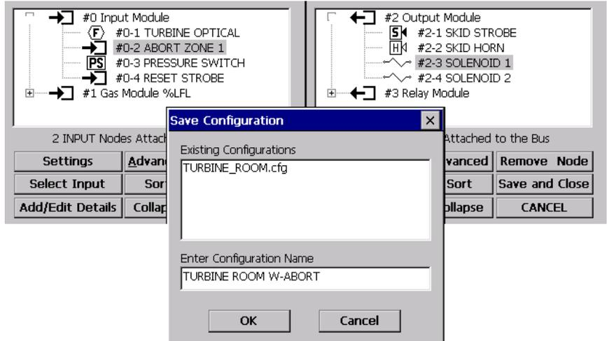
FIGURE 14.2. Naming the configuration.
