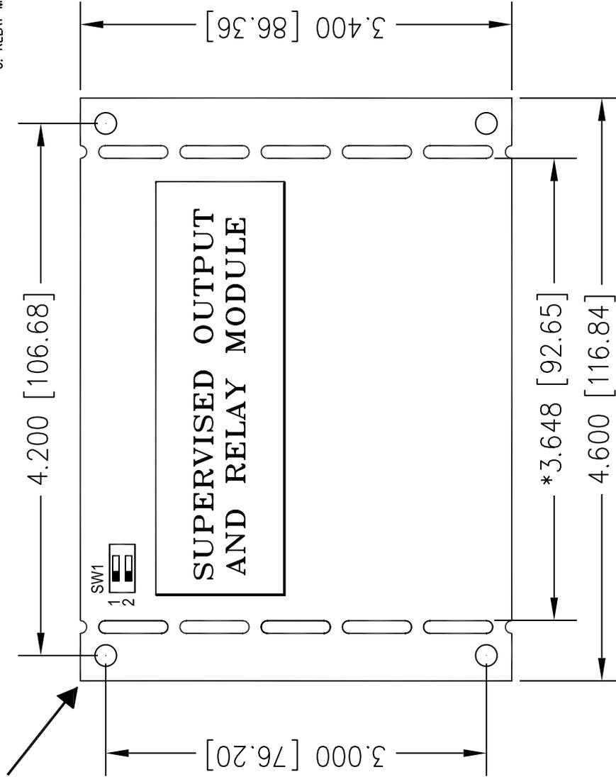
MODEL FG8800-1705 SUPERVISED OUTPUT MODULE, 1725 RELAY MODULE
