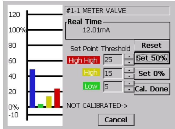
FIGURE 10.4 SET SPAN menu with 20.01 mA applied to same input.
