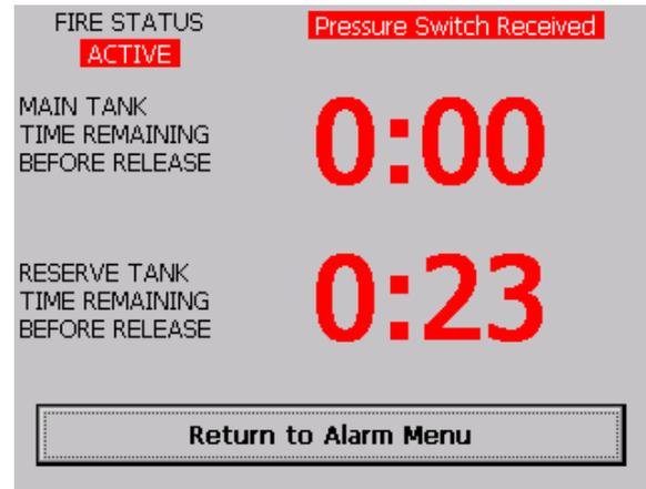
FIGURE 16.6 Pressure switch monitor
