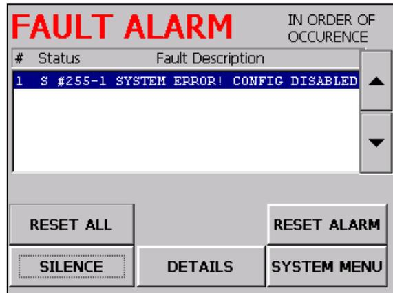
FIGURE 24.2 A fault alarm is created. Reoccurring alarms will appear every 30 minutes unless further action is taken.
