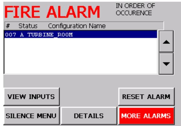
FIGURE 22.1 Viewing the fire alarm menu when another alarm arrives.
