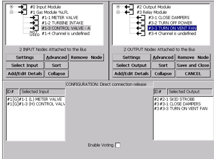
FIGURE 15. Direction connection from gas to relay node.
