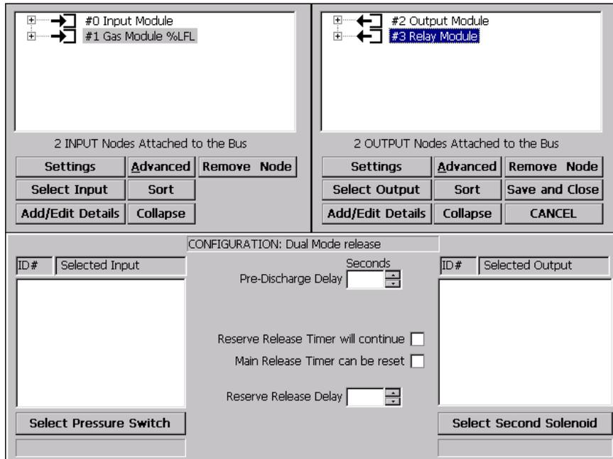
FIGURE 16. Dual release menu - preparing to configure.
