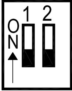
IMPORTANT: OBSERVE THE "ON" POSITION PRIOR TO SLIDING THE CONTACT POLE. SW1 IS ORIENTED DIFFERENTLY ON DIFFERENT MODULES. VERIFY THE CONTACT SLIDE IS NOT "PARTIALLY" MOVED.
