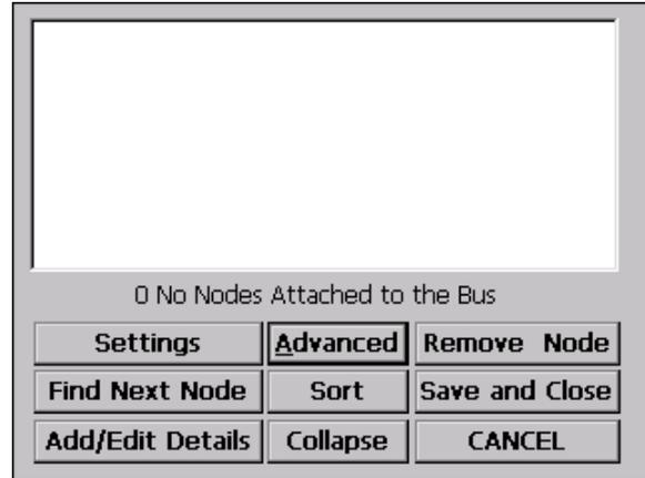
FIGURE 5.3 Ready to search nodes. NOTE: Only buttons pertaining to the startup procedure will appear until the first node is discovered and located in the above menu.
