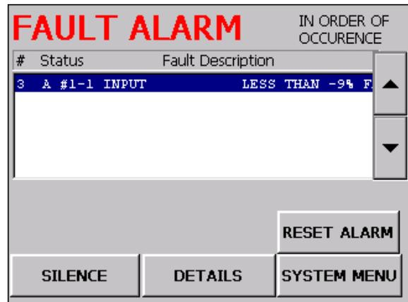
FIGURE 15.10 Fault alarm screen
