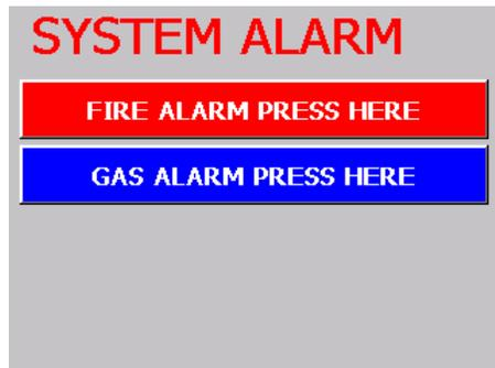
OPERATOR HAS THE CHOICE OF WHICH INCOMING ALARM TO INVESTIGATE FIRST. FAULT AND WARNING ALARMS ARE ALSO INDICATED HERE. IF THIS MENU IS NOT ATTENDED TO THE SYSTEM WILL AUTOMATICALLY EXECUTE ITS PROGRAMMING AS IT WAS SET UP TO.
