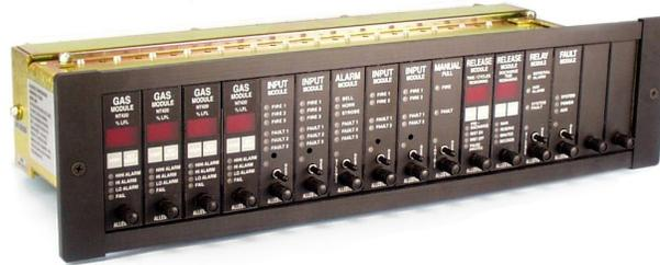
A protection circuit monitors the power supply voltage for under or over voltage inputs. Should the power supply voltage deviate from its required specification, the system fault LED will illuminate and the sonalert will sound, followed by the relay changing state.
